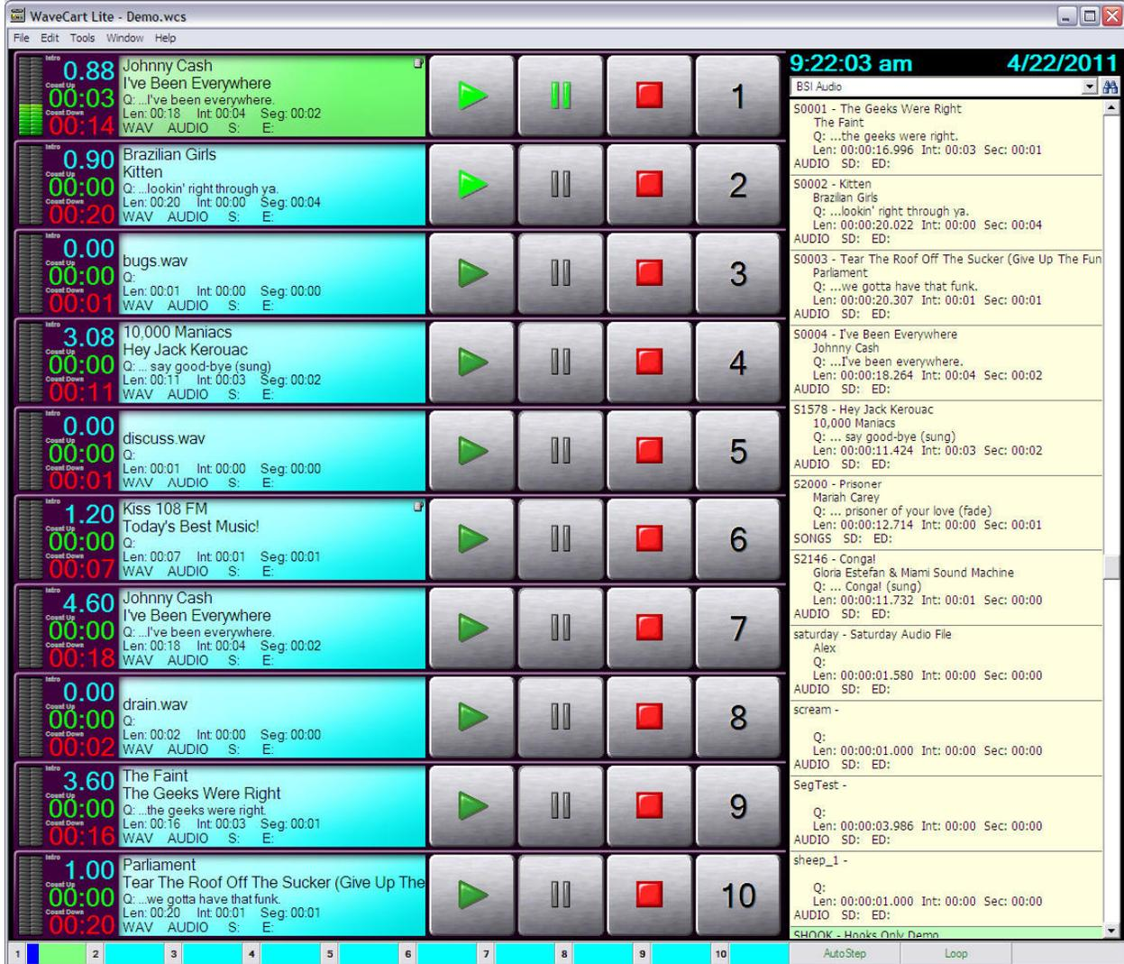
WaveCart uses a standard PC and sound-card to play back multiple audio files, optionally to different audio outputs and can automatically sequence from one deck to another.
